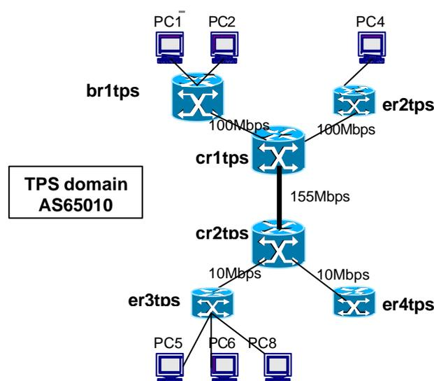
*Figure 6-1. Trial topology for single-domain network scenario. PC1-PC8 – traffic generators/analyzers*
