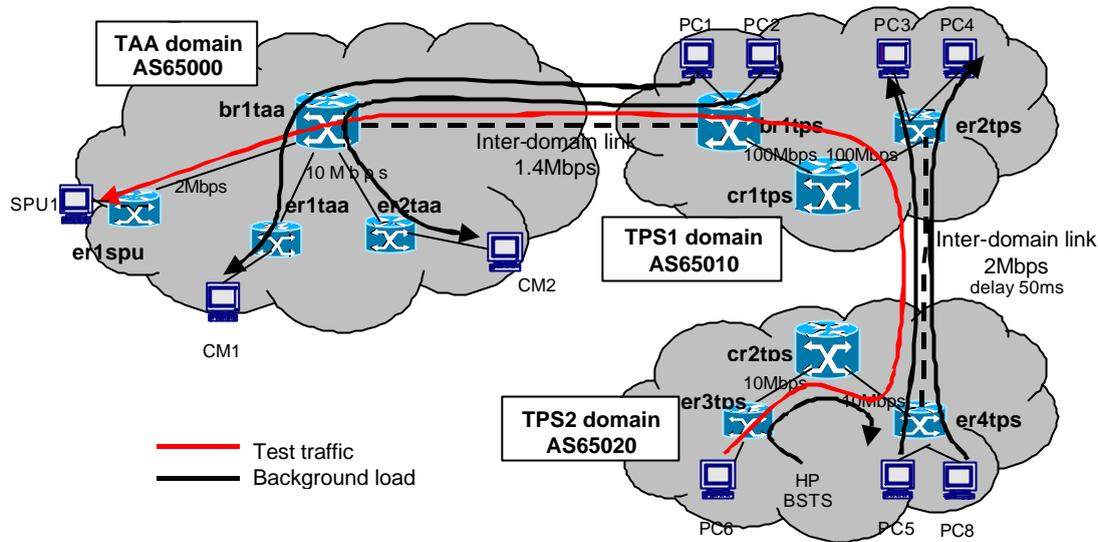
**Figure 6-10. Trial topology for inter-domain network scenario**
