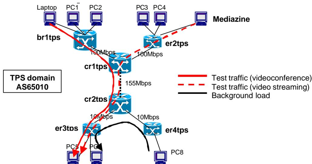
Figure 7-5. Trial topology in Mediazine tests.
