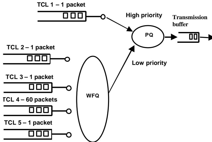
*Figure 6-9. Router output port architecture for PMM service*
