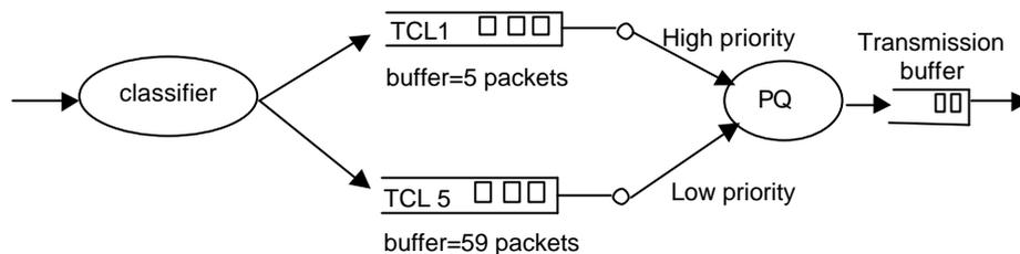
**Figure 6-3. Architecture of router output port in TCL1 trials**
