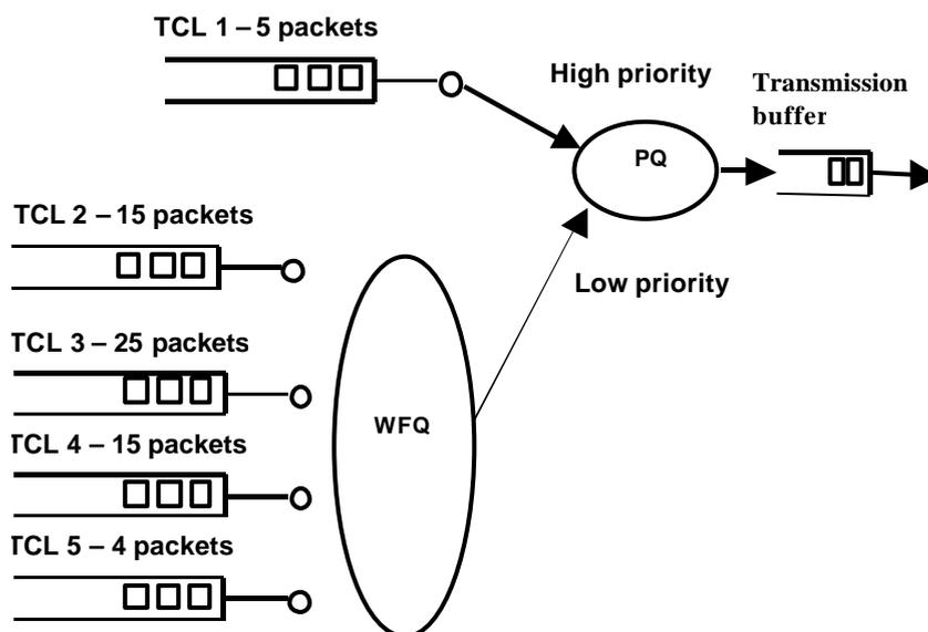
**Figure 6-7. Router output port architecture for PMM service**
