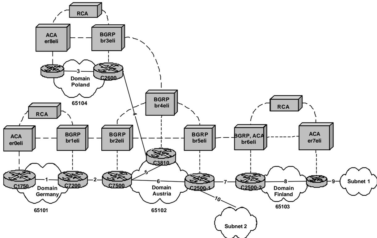
Figure 10-6. Inter-domain testbed for signalling
