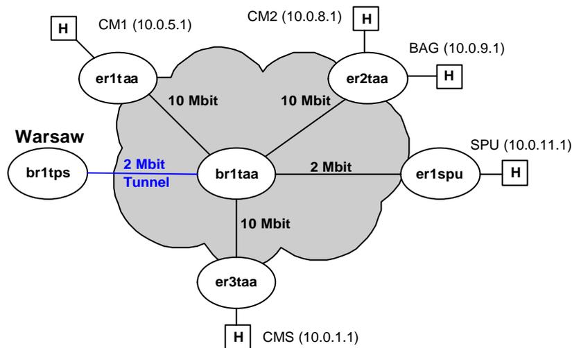
Figure 9-1. Link capacity in the Vienna network topology
