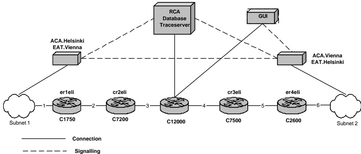
Figure 10-5. Intra-domain testbed for signalling
