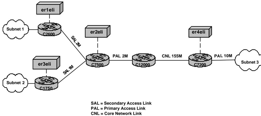
Figure 10-7. Secondary access link testbed
