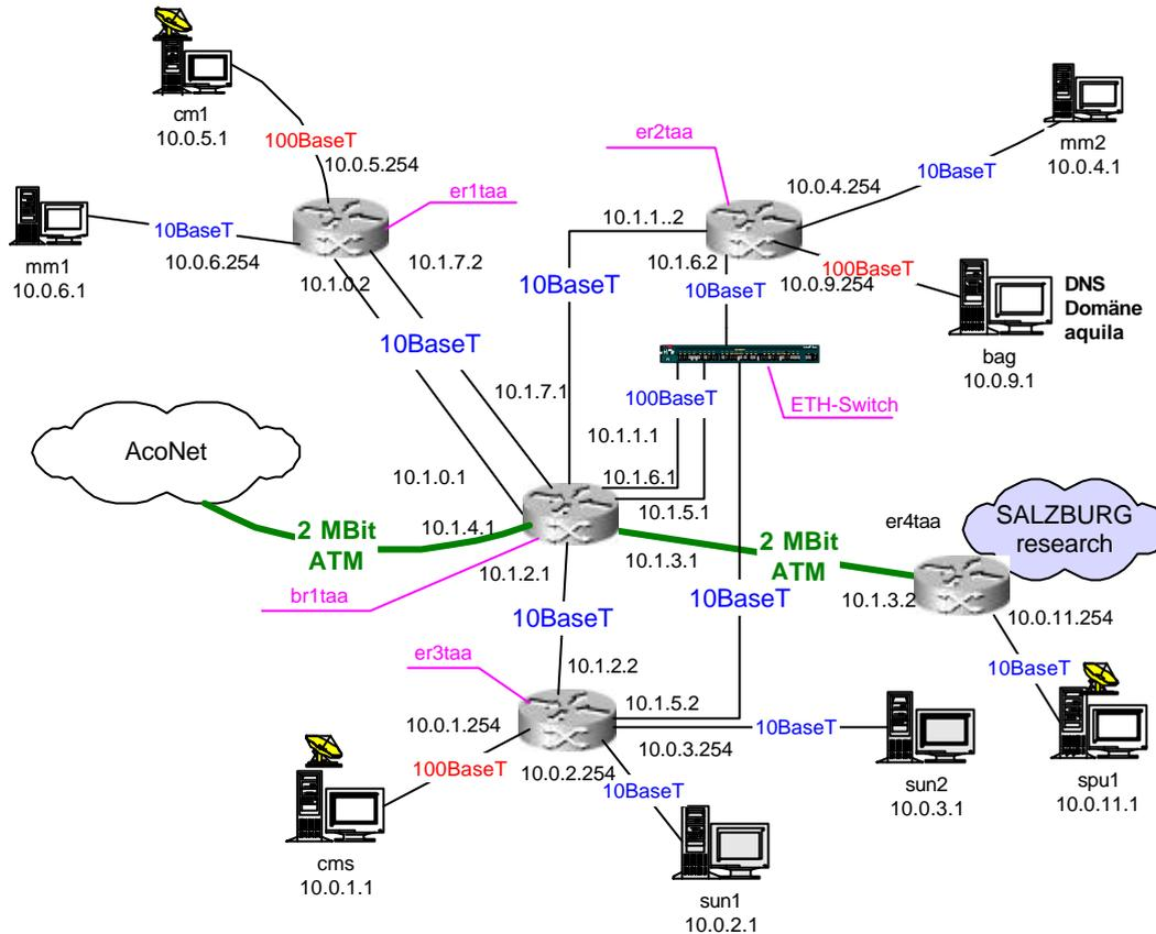
**Figure 10-3. TAA testbed for the 2<sup>nd</sup> trial**
