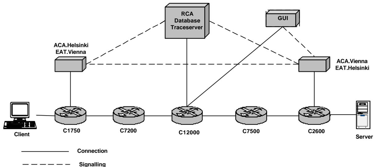
*Figure 8-1. Intra-domain scenario test network*
