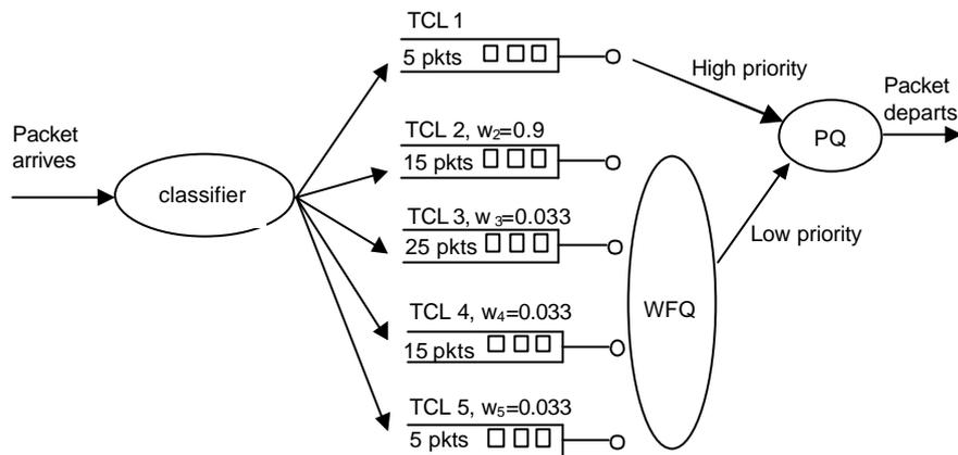
**Figure 6-5. Architecture of router output port in TCL2 trials**
