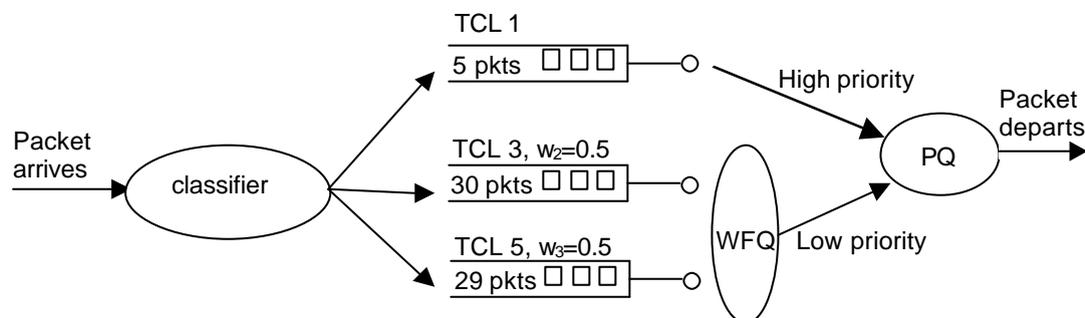
**Figure 6-11. Architecture of router output port on the inter-domain link**
